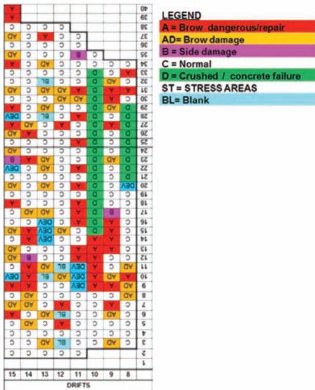
Figure 9—Structural condition of West Cave drawpoints by November 2011
