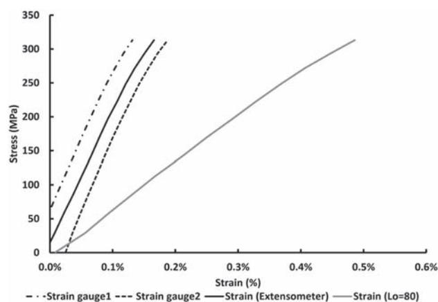
Figure 6—A schematic diagram of the stress strain curve in the elastic region, showing the expected Young's modulus value and the values calculated and recorded from the tensile tests conducted
