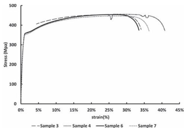
Figure 4—Stress-strain curve obtained from the 100 kN Schenck (Hydropuls PSA). Strain was calculated as change in displacement over  $L_o = 80$  mm
