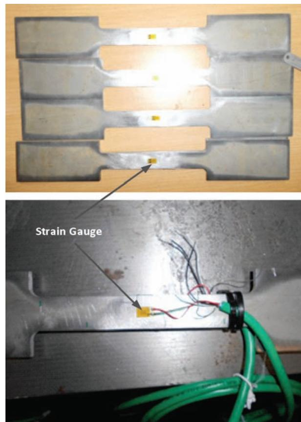
Figure 2 – Test specimen after strain gauging and attaching the Somat cables
