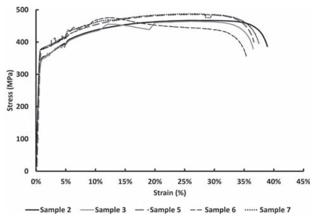
Figure 3—Stress-strain curve of TM 380 obtained from the I400 kN Instron (Model: 1344)
