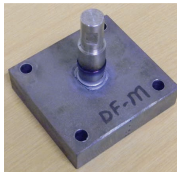
Figure 3—Completed FHPP weld
