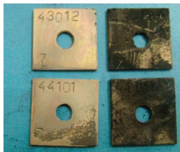
Figure 6—Photograph of Type 430 (upper row) and 441 samples (lower row) after exposure for 30 days. The samples on the left-hand side were cleaned
