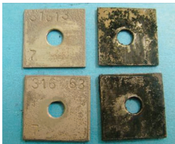
Figure 5—Photograph of Type 316L (upper row) and 316Ti samples (lower row) after exposure for 30 days. The samples on the left-hand side were cleaned
