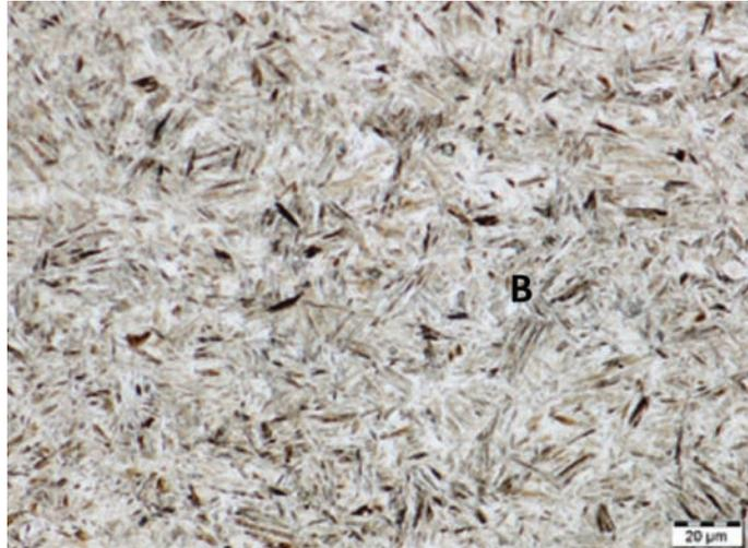
Figure 7—Microstructure of BN1 at a cooling rate of 30°C per second showing bainite (B) and martensite (M)
