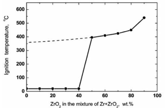
Figure 16—Addition of ZrO<sub>2</sub> increases the MIT of Zr<sup>42</sup>
