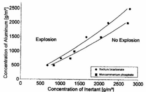
Figure 17—Inerting of aluminium powder<sup>46</sup>
