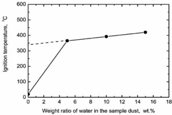
Figure 14—Effect of moisture on the ignition temperature of zirconium powder<sup>42</sup>
