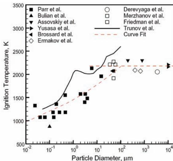
Figure 10—Influence of particle size on the MIT of aluminium<sup>40</sup>
