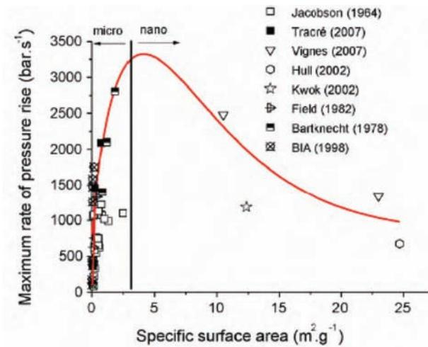
Figure 7—Effect of moving to nano-sized particles on pressure rise for aluminium powder<sup>22</sup>
