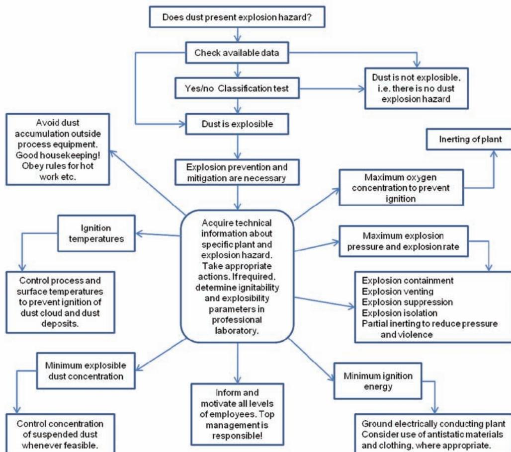
Figure 20—A summary of the approach to preventing dust explosions (redrawn from reference<sup>12</sup>)
