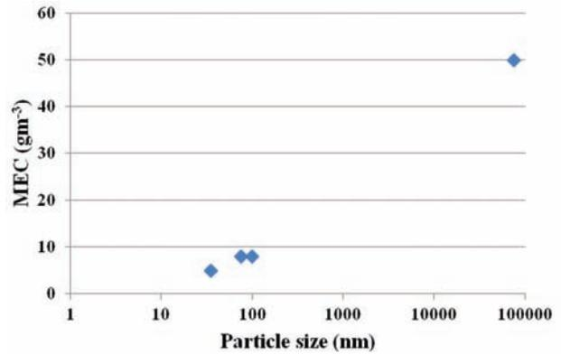
Figure 8—Effect of aluminium powder particle size on the minimum explosion concentration (redrawn from reference<sup>26</sup>)
