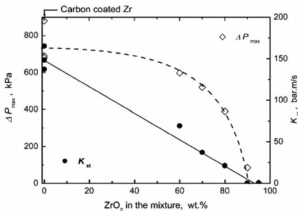
Figure 15—Effect of addition of ZrO<sub>2</sub> on the K<sub>st</sub> value of zirconium<sup>42</sup>
