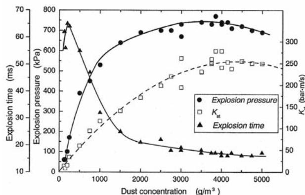
Figure 11—Dust deflagration index for tantalum as a function of the dust concentration<sup>31</sup>
