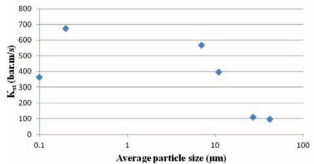
Figure 13—Influence of particle size on the dust deflagration index of aluminium (data from<sup>21,22</sup>)
