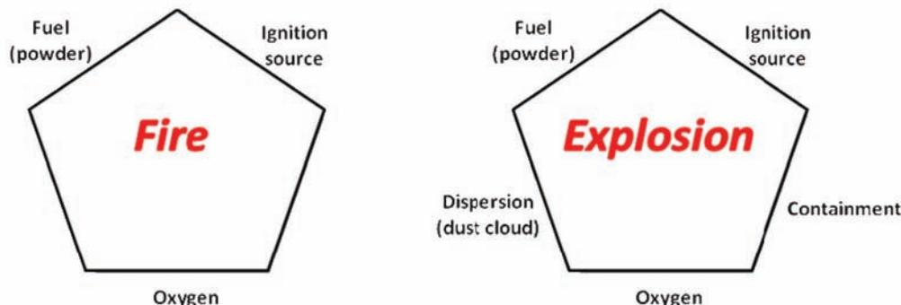
Figure 2—Schematic outline of the parameters for a fire or explosion (redrawn from reference<sup>8</sup>)
