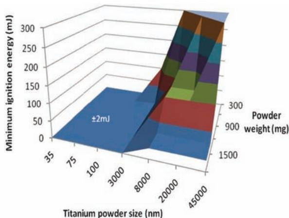
Figure 9—The dependence of the MIE of titanium on particle size and powder quantity (redrawn from reference<sup>32</sup>)
