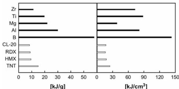
Figure 4—Comparison of combustion enthalpies of various materials<sup>11</sup>
