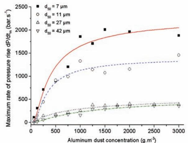
Figure 6—Effect of average aluminium powder size on the rate of pressure rise at different concentration levels<sup>21</sup>
