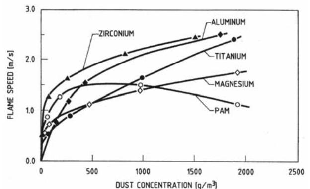
Figure 5—Flame speeds for various powders as a function of dust concentration<sup>12</sup>. Median powder sizes: ~45  $\mu\text{m}$  (Zr), ~9  $\mu\text{m}$  (Al), ~50  $\mu\text{m}$  (Ti), ~45  $\mu\text{m}$  (Mg)
