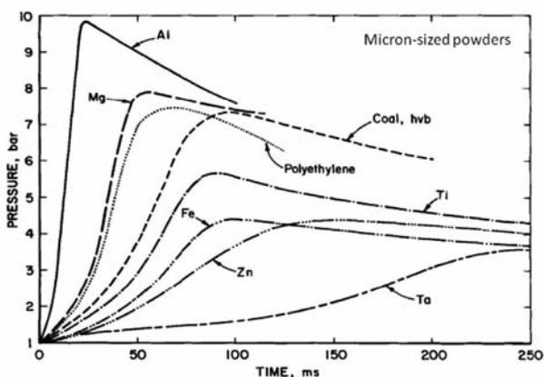
Figure 3—Comparison of energy release during controlled explosion tests of different powders<sup>10</sup>
