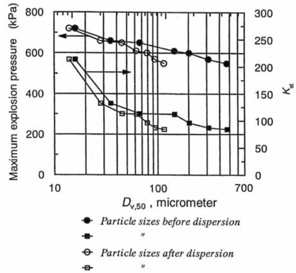
Figure 12—Influence of tantalum particle size on the K<sub>st</sub> value<sup>31</sup>
