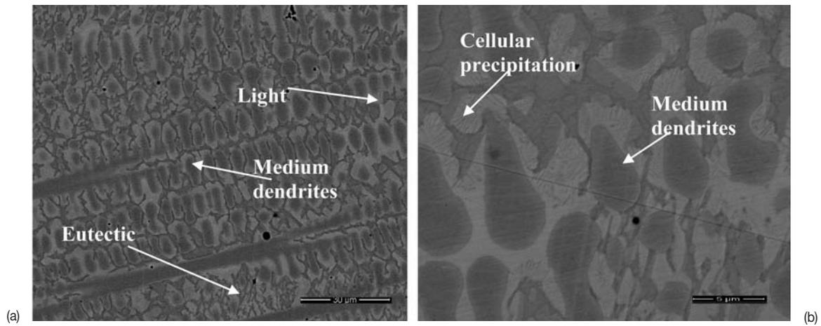
Figure 2—(a) SEM-BSE image of Alloy 2 showing medium grey dendrites ( $\sim\text{Pt}_2\text{V}$ ), a light phase  $\sim\text{Pt}_5\text{Al}_3$ , and a eutectic ( $\beta + \sim\text{Pt}_5\text{Al}_3$ ). Scale bar is 30  $\mu\text{m}$ . (b) SEM-BSE image of Alloy 2 showing medium grey dendrites ( $\sim\text{Pt}_2\text{V}$ ), a light phase ( $\sim\text{Pt}_5\text{Al}_3$ ) and solid state cellular precipitation. Scale bar is 5  $\mu\text{m}$
