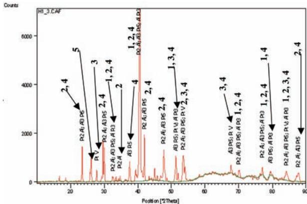
Figure 9—XRD pattern of Alloy 1H, average overall composition Pt-26.2Al-9.1V (at.%). Key: ~Pt<sub>3</sub>Al - 1, ~Pt<sub>2</sub>Al - 2, ~PtV - 3, ~Pt<sub>5</sub>Al<sub>3</sub> - 4, CaCO<sub>3</sub> - 5
