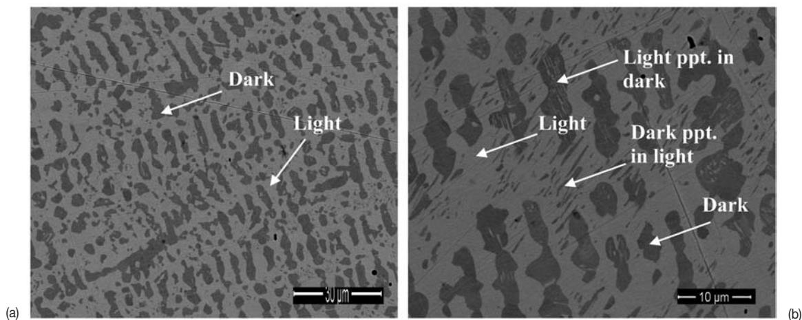
Figure 10—(a) SEM-BSE image of annealed Alloy Pt-21.1Al-17.1V (at.%) showing a dark phase (~PtV), a light phase (~Pt<sub>2</sub>Al) and dark precipitates in the light phase. Scale bar is 30 μm. (b) SEM-BSE image of annealed Alloy Pt-21.1Al-17.1V (at.%) showing a dark phase, a light phase, a eutectic, and a possible light precipitates in the dark phase. Scale bar is 10 μm
