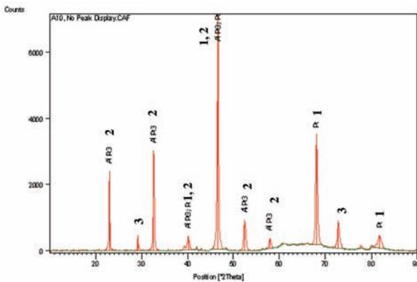
Figure 7—XRD pattern of as-cast Alloy 6, average overall composition Pt-6.0Al-10.1V (at.%). Key: (Pt) - 1, ~Pt<sub>3</sub>Al - 2, and CaCO<sub>3</sub> - 3 in the resin mounting
