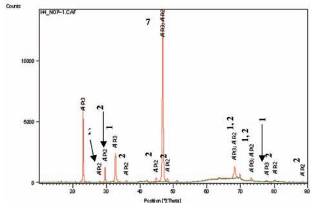
Figure 12—XRD pattern of alloy 5H, average overall composition Pt-23.2Al-7.1V (at.%). Key: ~Pt<sub>3</sub>Al – 1 and ~Pt<sub>2</sub>Al – 2
