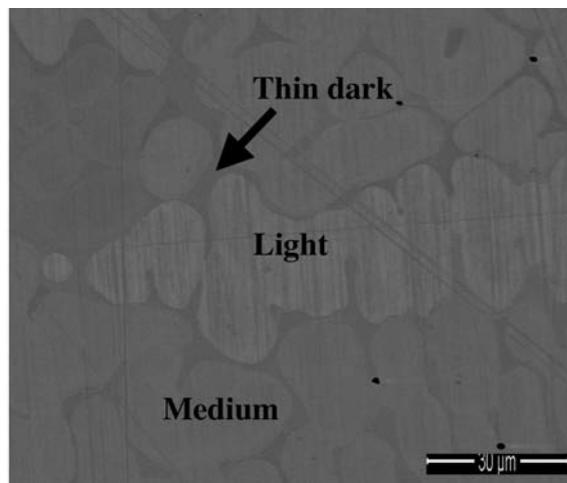
Figure 5—SEM-BSE image of as-cast Alloy Pt-22.3Al-7.9V showing a light grey phase (~Pt<sub>3</sub>Al), a medium grey phase (~Pt<sub>3</sub>Al) and a thin dark grey phase (~Pt<sub>2</sub>Al). Scale bar is 30 μm
