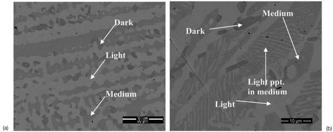
Figure 11—(a) SEM-BSE image of annealed alloy Pt-10.8Al-25.5V (at.%) showing a medium grey phase (~Pt<sub>2</sub>V), a light phase (~Pt<sub>3</sub>Al), and a dark phase (~PtV). Scale bar is 30 µm. (b) Figure 11(b). SEM-BSE image of annealed alloy Pt-10.8Al-25.5V (at.%) showing a medium grey phase (~Pt<sub>2</sub>V), a light phase (~Pt<sub>3</sub>Al), a dark phase (~PtV), and 2-phase dendrites. Scale bar is 10 µm
