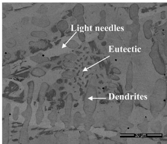
Figure 1—SEM-BSE image of Alloy Pt-26.6Al-9.1V (at.%) showing medium grey dendrites ( $\sim\text{Pt}_3\text{Al}$ ) with a dark thin layer ( $\sim\text{Pt}_3\text{V}$ ), light needles ( $\sim\text{Pt}_5\text{Al}_3$ ), and a eutectic. Scale bar is 30  $\mu\text{m}$
