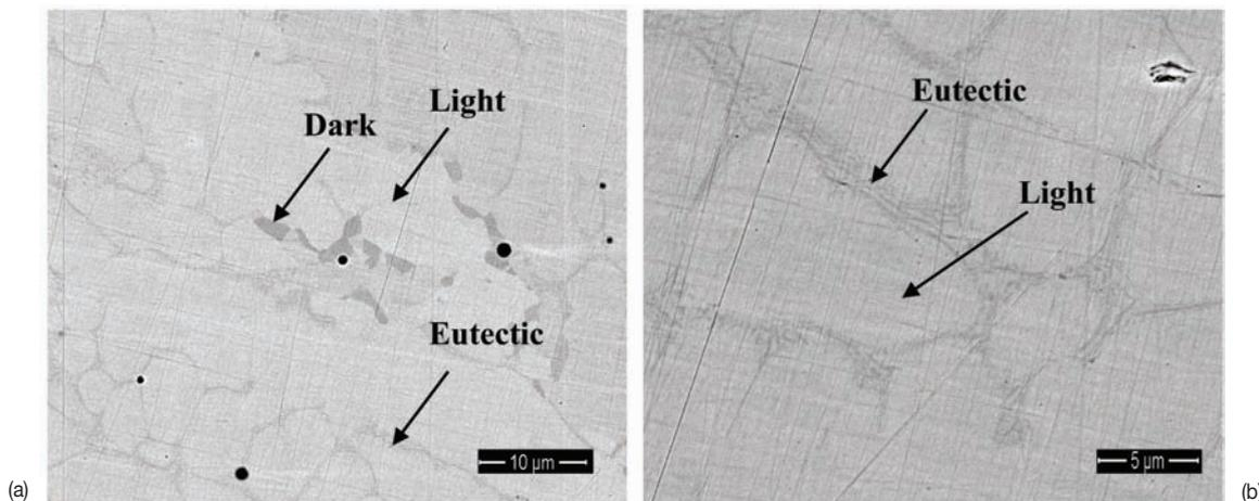
Figure 13—(a) SEM-BSE image of annealed alloy Pt-5.8Al-10.3V (at.%) showing a light grey phase (Pt), a dark phase ( $\sim$ Pt<sub>2</sub>V), and a eutectic. Scale bar is 10  $\mu$ m. (b) SEM-BSE image of annealed alloy Pt-5.8Al-10.3V (at.%) showing a light grey phase, and a eutectic at a higher magnification (x 10 000). Scale bar is 5  $\mu$ m
