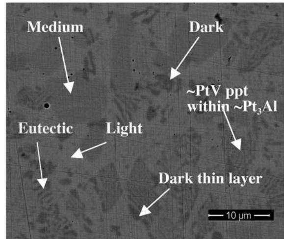
Figure 8—SEM-BSE image of annealed alloy Pt<sub>64.7</sub>Al<sub>26.2</sub>V<sub>9.1</sub> (at.%) showing a medium grey phase, a light phase, a dark phase, a eutectic, and dark precipitate the within medium grey phase. Scale bar is 10 μm
