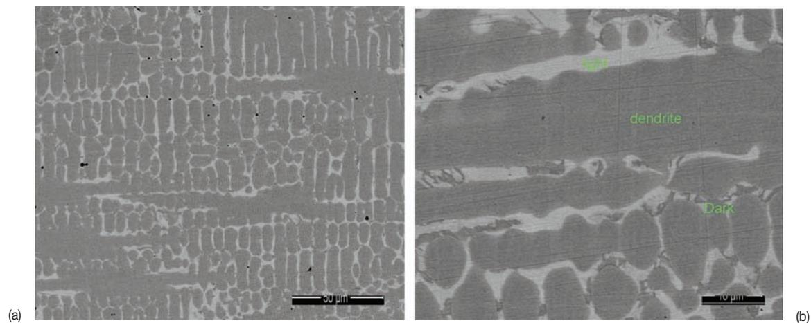
Figure 3—(a) SEM-BSE image of as-cast Alloy Pt-9.6Al-21.1V (at.%) showing dendrites ( $\sim\text{Pt}_3\text{V}$ ) and a light phase ( $\sim\text{Pt}_3\text{Al}$ ). Scale bar is 50  $\mu\text{m}$ . (b) SEM-BSE image of as-cast Alloy Pt-9.6Al-21.1V (at.%) dendrites ( $\sim\text{Pt}_3\text{V}$ ), a light phase ( $\sim\text{Pt}_3\text{Al}$ ) and a dark phase ( $\sim\text{Pt}_2\text{Al}$ ) between the dendrites. Scale bar is 10  $\mu\text{m}$
