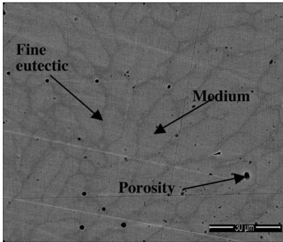
Figure 6—SEM-BSE image of as-cast Pt<sub>83.9</sub>Al<sub>6</sub>V<sub>10.1</sub> (at.%) showing a medium grey phase (Pt), a fine eutectic ((Pt) + ~Pt<sub>3</sub>Al) and porosity (dark spots). Scale bar is 30 μm
