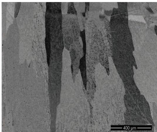
Figure 4—SEM-BSE image of as-cast Alloy Pt<sub>76.2</sub>Al<sub>17.4</sub>V<sub>6.4</sub> (at.%) showing a single phase (~Pt<sub>3</sub>Al) with grains at different orientations. Scale bar is 400 μm
