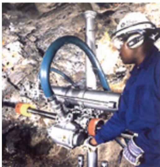
Figure 4—Boart Longyear Metre Eater. A pneumatic AQ/BQ drilling machine ( http://boartlongyear.virtual.vps-host.net:8080/web/guest/99 )
