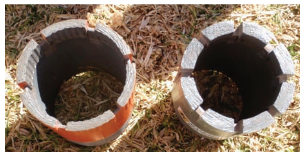
Figure 5—A thin (left) and standard (right) BX drilling bit (60 mm diameter)
