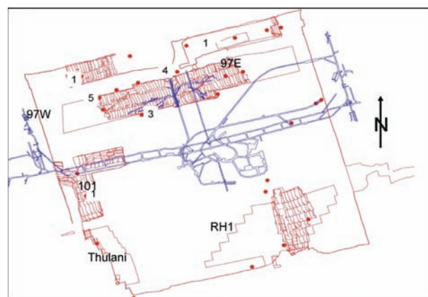
Figure 1—Showing position of major damage associated with seismic events numbers indicating injuries associated with the damage
