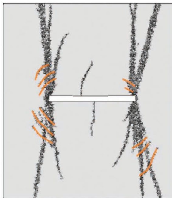
Figure 16—Fracture map from simulation of C17 at 220 MPa load, with curved fractures highlighted
