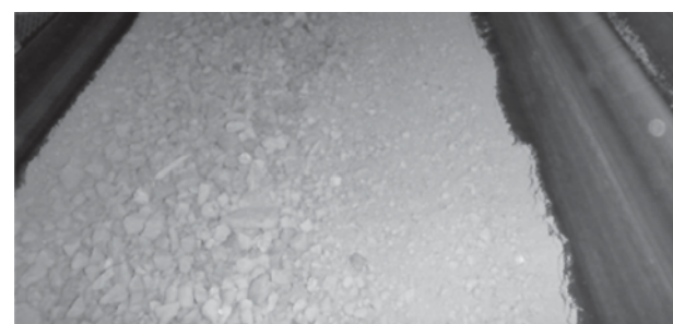
Figure 13—Feed size segregation on a conveyor belt
