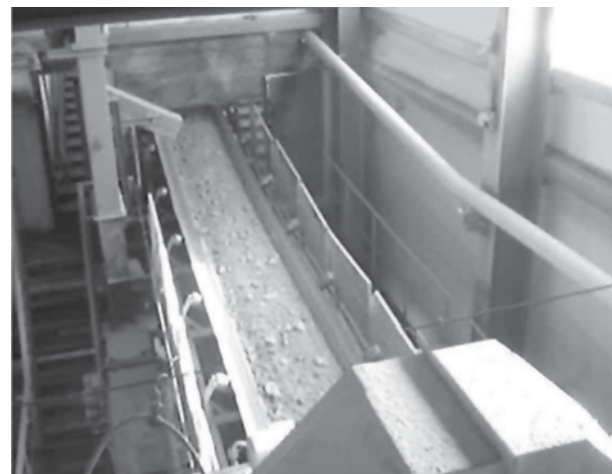
Figure 10—Flakes in the HPGR discharge at Vasilkovka
