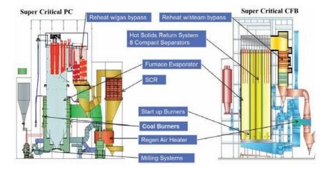
Figure 2-Comparison of the features of the largescale OTSC PC and OTSCCFB
