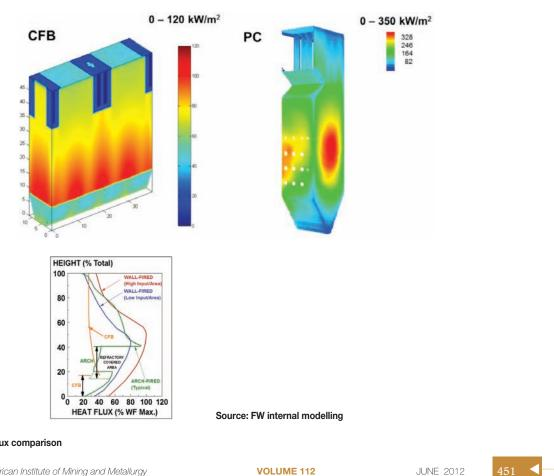
Figure 3–CFB vs. PC heat flux comparison
