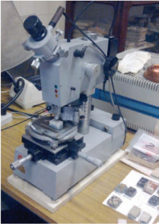
Figure 1 – The Leitz micro-durimeter (Model Durimet 2) employed to perform the Knoop test
