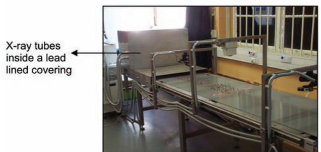
Figure 4—XRT monitor setup showing position of X-ray tubes
