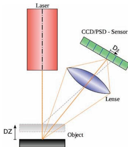
Figure 1—Principle of laser triangulation
