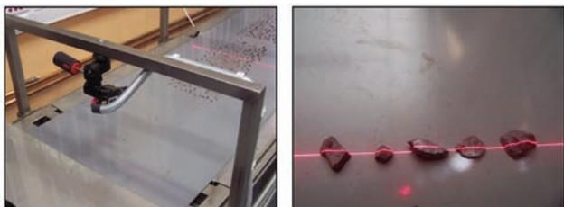
Figure 5—X-ray monitor showing particles along laser beam
