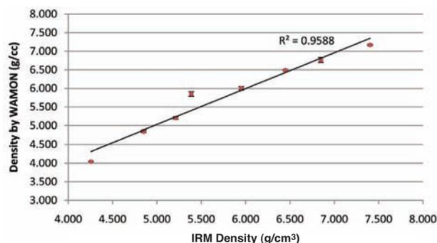
Figure 11—The validation results using F-samples plotted to 95% confidence limits
