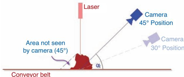
Figure 2—Laser and camera alignment
