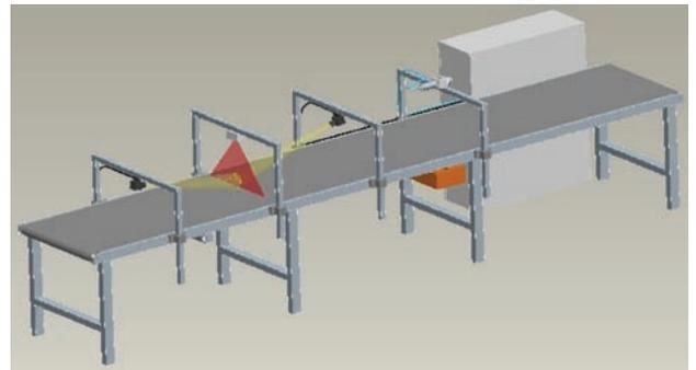
Figure 3—Schematic layout of optical cameras on conveyor belt
