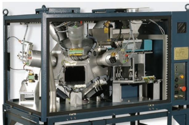
Figure 2—The VSFD device used to create 3D models of particles
