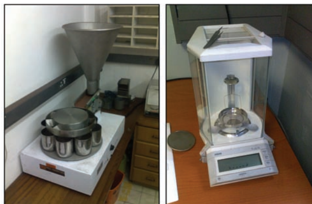
Figure 3—The samples were split using a spinning riffler (left) and weighed on a micro balance (right)
