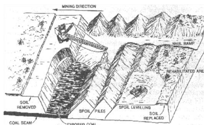
Figure 3—Strip mining with concurrent rehabilitation (after Wells et al. 8 )
