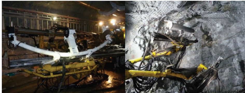
Figure 9—A 2,3 m wide handler mounted on a twin boom jumbo (left) and a MESHA® installation handler mounted on a jumbo boom picks up the roll of mesh auto-matically (right)
