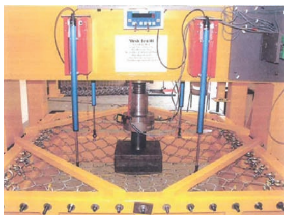
Figure 4—Measured forces in the anchorages for the 5 mm wire diameter heavy mild steel chain-link mesh
