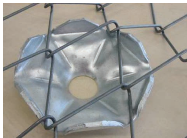
Figure 2—Specially designed spike plates for the underground system
