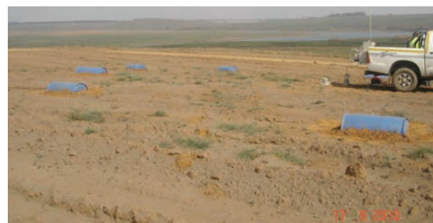
Figure 1—A typical sampling arrangement, with six half-barrel collectors feeding to a central manifold. Mine topsoiled and rehabilitated
