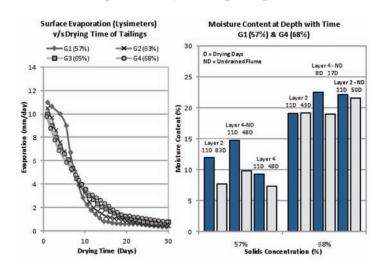
Figure 6-Summary of fixed flume (KP) lysimeter data and prolonged moisture contents
