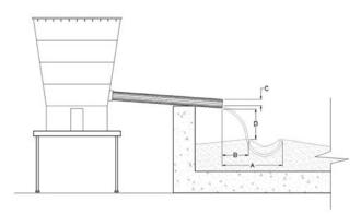
Figure 4-Discharge arrangement and measurement in both flumes
