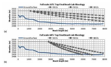
Figure 10–Predicted beach profiles (a) 63% and (b) 68% solids, top final beach
