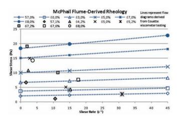
Figure 8-Flume-derived rheological results and interpolated laboratory rheology
