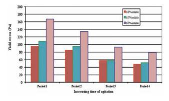
Figure 4—Influence of agitation-induced shear thinning on the yield stress
