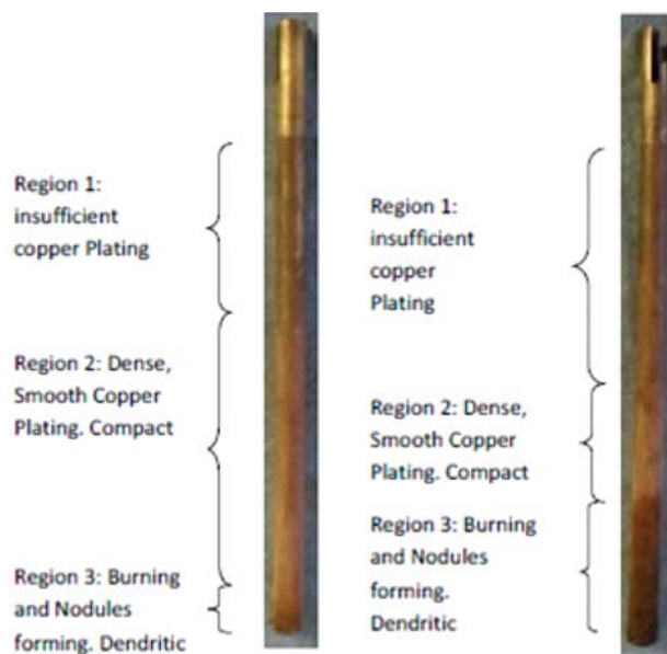
Figure 10—Optical view of copper cathode after electrolysis showing morphological regions
