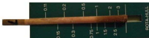
Figure 8—Photo showing the relative current densities and copper cathode after electrolysis
