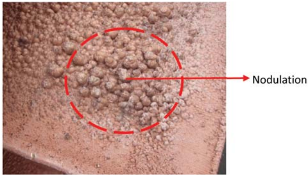
Figure 1—Cathode showing nodulation on the cathode surface
