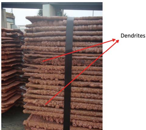
Figure 3—Cathode showing dendrites on the edges of the cathode
