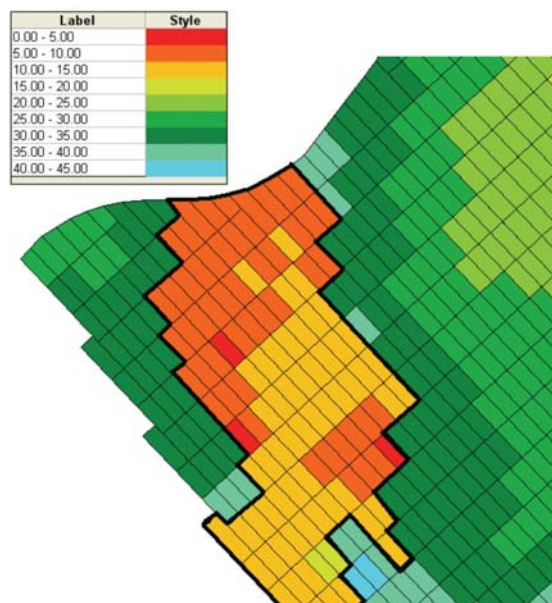
Figure 9—No. 5 seam overburden depth 6
