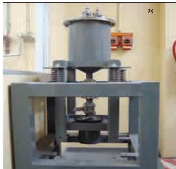
Figure 4—Photographic representation of Mintek's roller mill—(a) mill drum on the two driving rolls, (b) discharge frame
