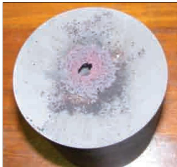
Figure 5—Material blown out of the crucible
