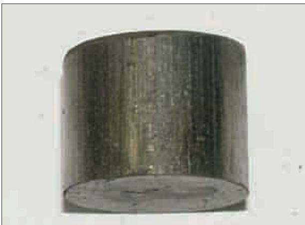
Figure 4—Typical green compact after uniaxial compaction
