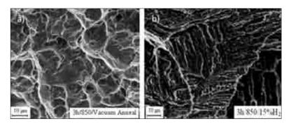
Figure 3—(a) Ductile-dimple fracture surface of vacuum annealed (850°C) specimen, (b) facetted brittle cleavage after 3h/850/15H<sub>2</sub> treatment
