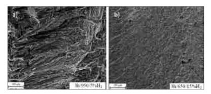
Figure 4—(a) Facetted quasi-cleavage after 3h/950/5H<sub>2</sub>, (b) fine granulated fracture surface appearance after 3h/650/15H<sub>2</sub>
