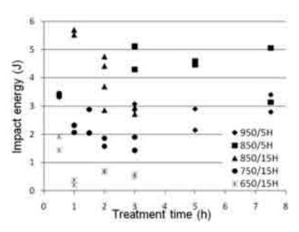
Figure 2—Impact energy as function of THP treatment
