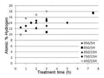
Figure 1—Hydrogen absorption as function of THP treatment condition
