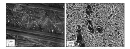
Figure 6—(a) Small spherical precipitates (light phase) visible within some martensite plates (3h/850/5H<sub>2</sub>), (b) Dense distribution of needle-like precipitates formed at 2h/650/15H<sub>2</sub>
