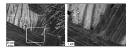
Figure 5—(a) Widmanstätten ( $\alpha$ + $\beta$ ) plate morphology evolved from the 950/5H<sub>2</sub> treatment, (b) higher magnification (see window in (a)) indicates fine precipitate (light phase) within some plates
