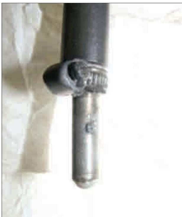
Figure 7—Blocked sonic nozzle
