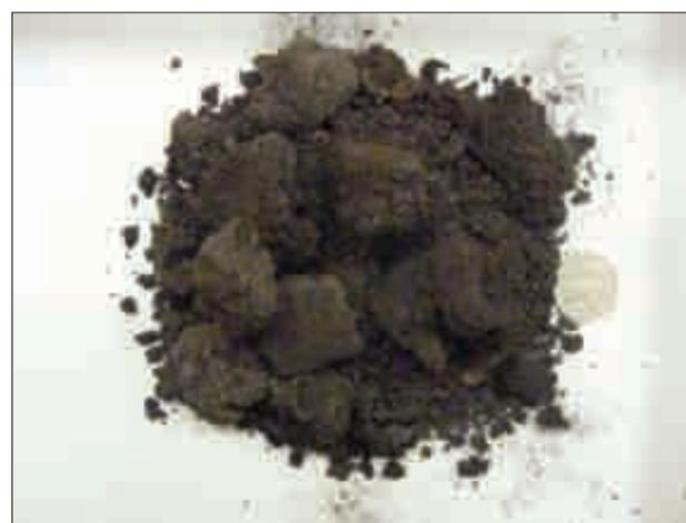
Figure 8—Metallothermally produced titanium product
