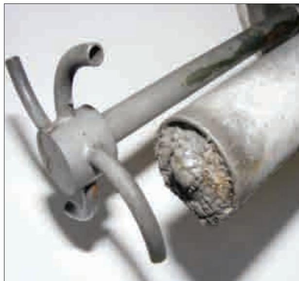
Figure 4—Blocked feed tube
