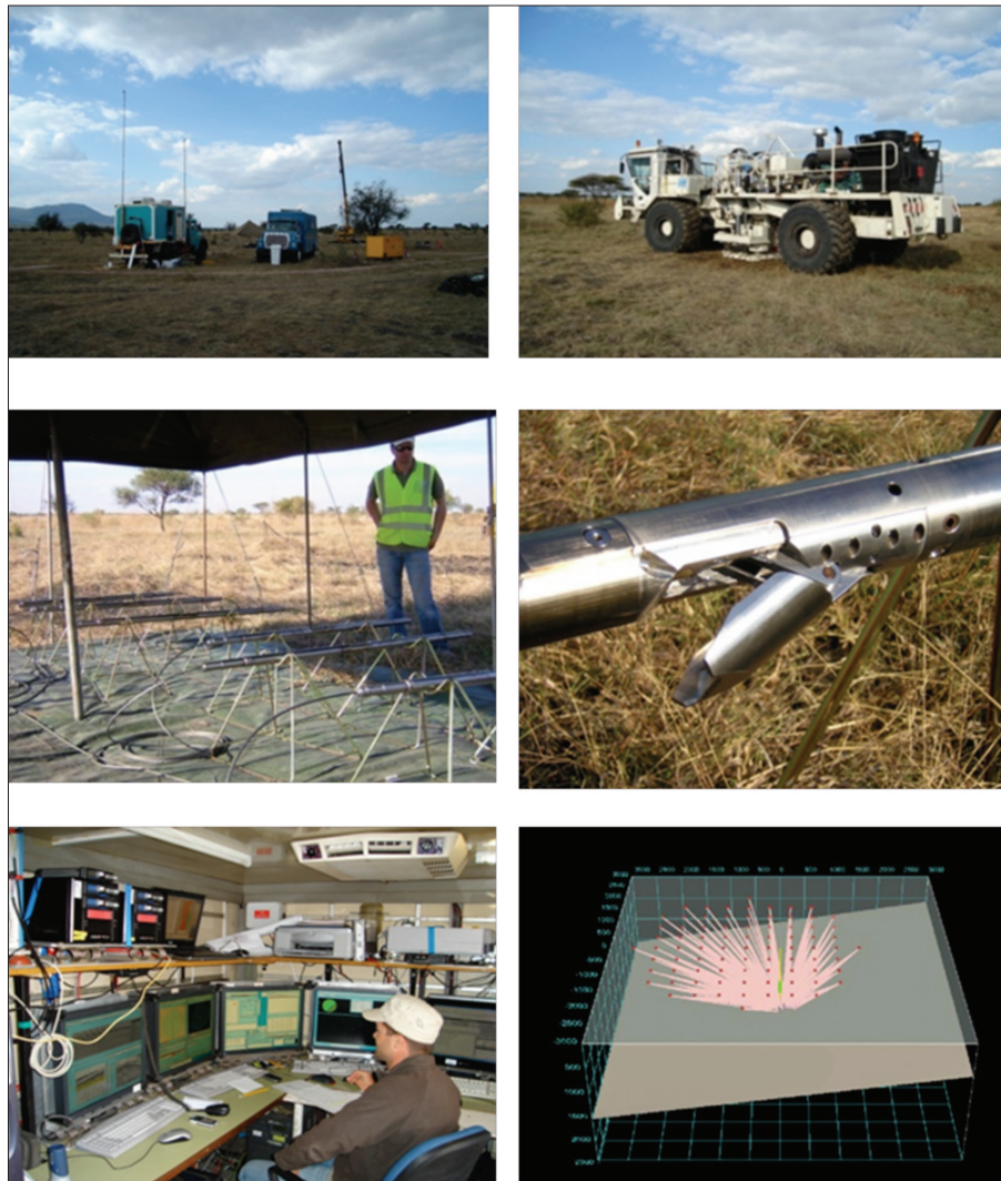
Figure 10—a) CGGV Seismic recording truck (foreground), Weatherford borehole geophysical logging truck (middle) and crane for VSP tool deployment (background); b) CGGV Nomad 65 Vibrator; c) 6 levels of CGGV/Sercel SlimWave tool ready for deployment; d) sidewall calliper brace on SlimWave element in open position; e) Engineer inside CGGV seismic recording truck; f) Survey simulation and design using 3D raytracing (VSFusion)
