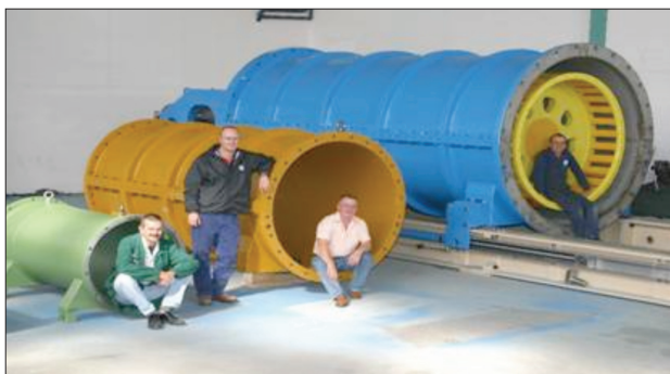
Figure 8—Photograph illustrates the scale-up of IsaMill™ technology; M1000, M3000 and M10000 mills: M3000 initially at Mt Isa Mines (1995), and the first M10000 at Anglo Platinum's WLTR plant (2003)
