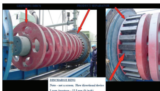
Figure 2—Layout and Internal arrangements of a large-scale IsaMill**
