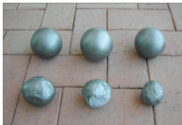
Figure 10—Effect of the discharge modification on the balls
