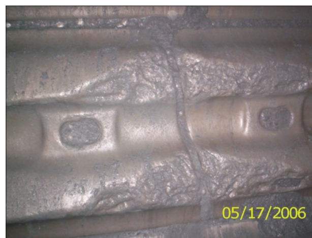
Figure 11—Effect of the discharge modification on the liners
