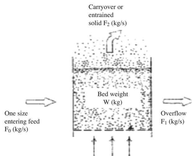
Figure 5—Representation of the roaster flow material balance<sup>2</sup>
