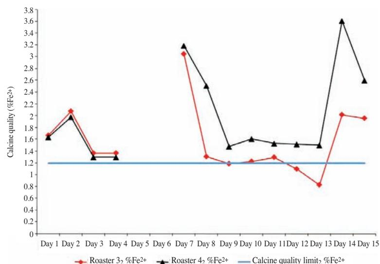
Figure 7—Results of semi-industrial scale roast test work. The test was performed at 950°C and O<sub>2</sub> in the fluidizing air in roaster 3 was reduced by 60% to 22.8% on day 2 and roaster 4 maintained at 26%
