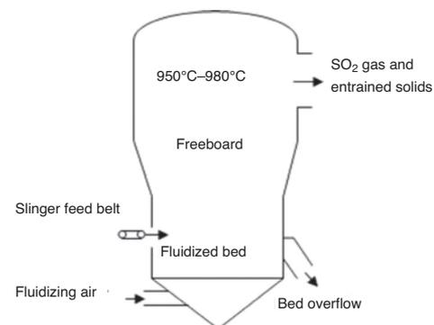
Figure 1—Representation of a typical Zincor fluidized roaster
