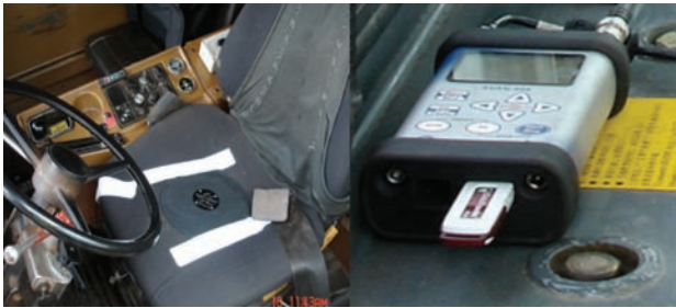
Figure 2—Dytran triaxial seat accelerometer (left) and SVAN958 HVM data acquisition system (right)
