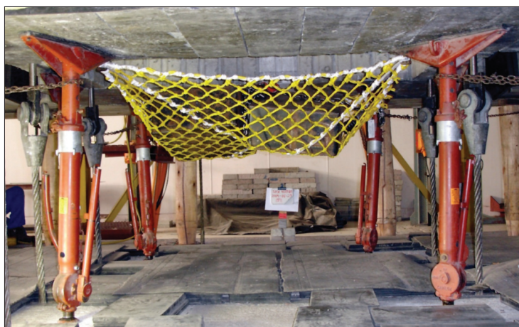
Figure 1—Safety net test at Savuka, showing the 450 kg twin drop mass arrested by the safety net. Note the diagonal and perimeter net reinforcement ropes attached to the Camlok prop hooks
