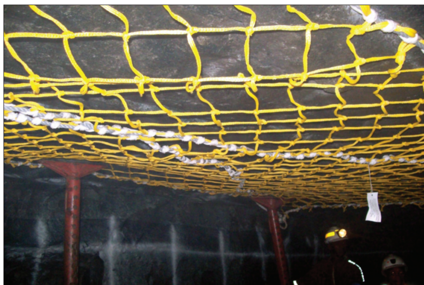
Figure 10—The same installation as in Figure 9 showing the Camlok props clamping the net front edge against the hangingwall at the stope face
