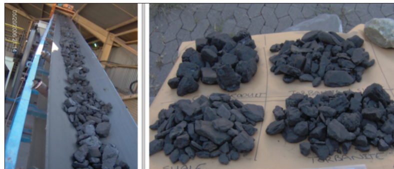
Figure 10—Coal, torbanite, and shale separation on an XRT sorter
