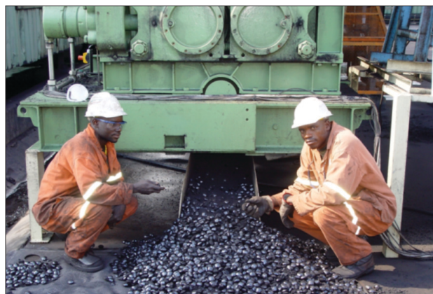
Figure 4—Briquetting press and binderless briquettes produced
