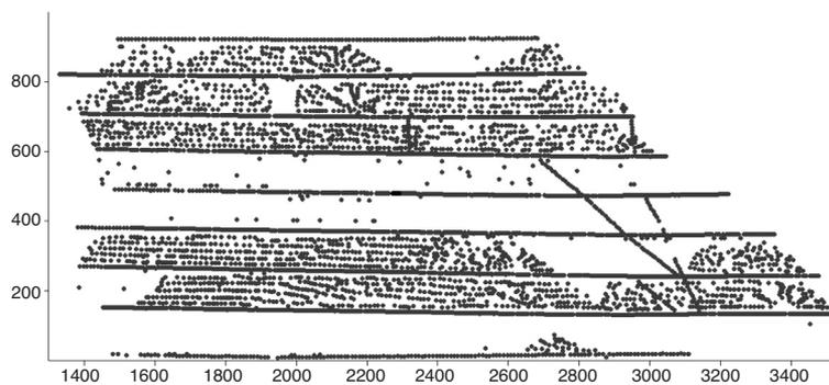
Figure 1—Post-plot of data used in case study, Geevor Tin Mine, Simms Lode
