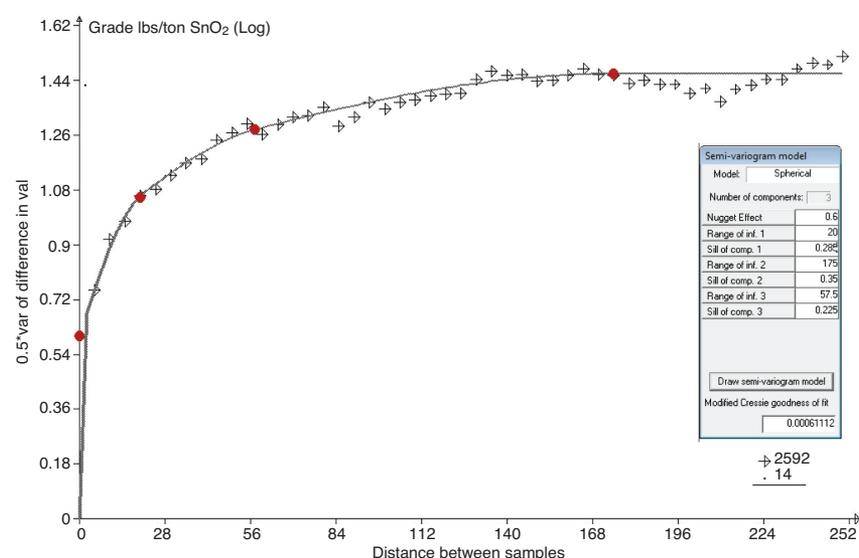
Figure 4—Semi-variogram for logarithm of tin grades in development drives, Simms Lode
