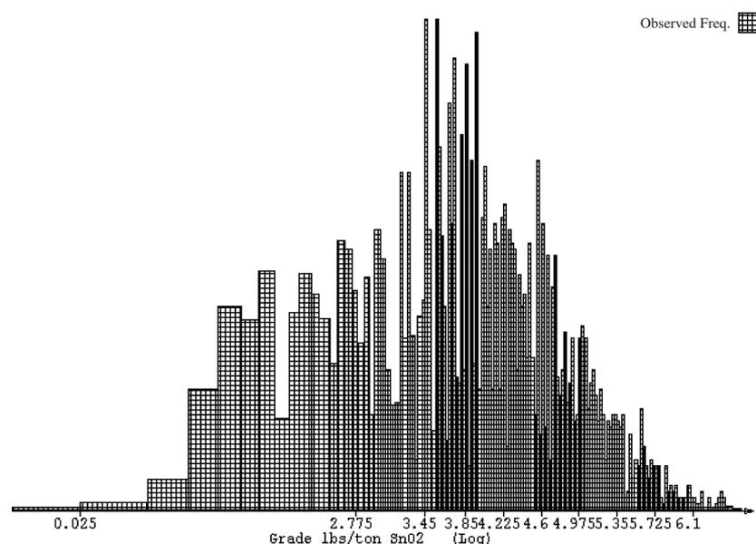
Figure 3—Histogram of logarithm of tin grades in development drives, Simms Lode
