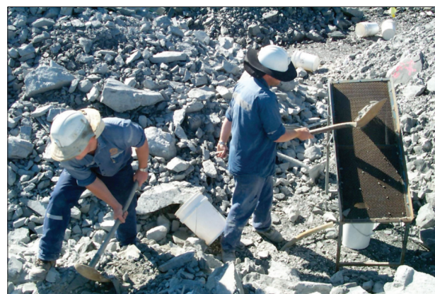
Figure 2—Collecting 50 kg 'grab' samples from a development stockpile using a portable -10 mm screen at the Bendigo mine site. Each white bucket held 25 kg of sample
