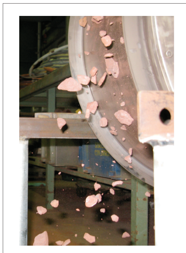
Figure 7—Photo of rocks leaving a drum. Approximate rotational speed was 4 rpm
