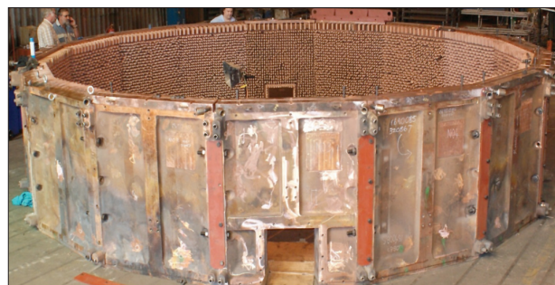
Figure 4—Shop assembly of the 12 MW DC furnace CFM sidewall cooling panels
