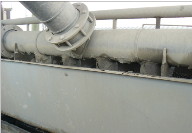
Figure 5—Typical feed manifold arrangement for wet drum magnetic separators
