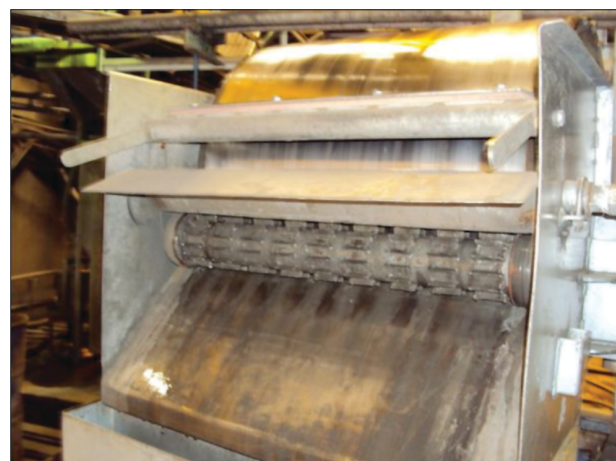
Figure 8—Rotary vane scraper system for magnetic concentrate removal (courtesy of Eriez Magnetics)
