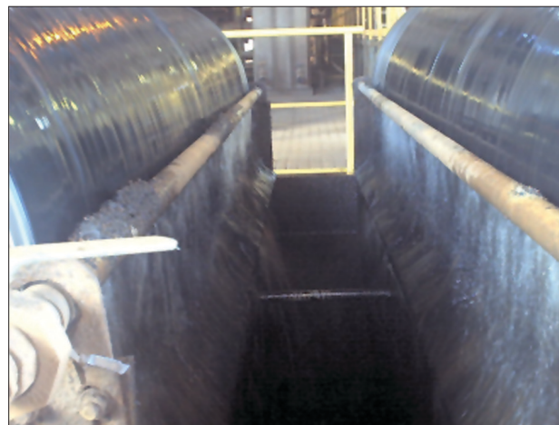
Figure 7—A spray water installation for the removal of magnetite concentrate
