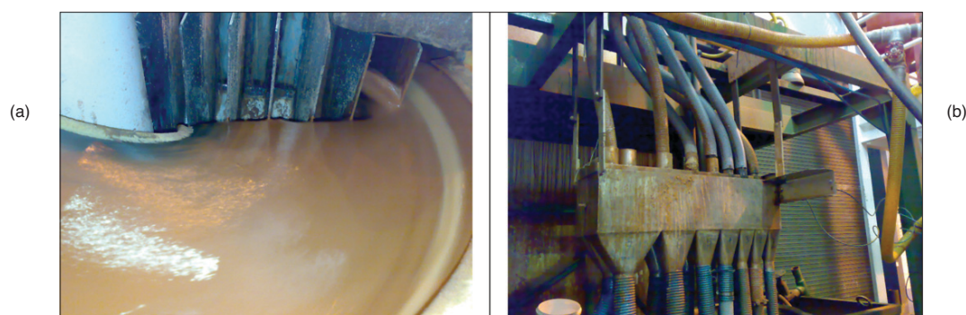
Figure 2—Components of the equipment set-up are depicted in the mouth-organ splitter (a) and the pneumatic sampling point (b)
