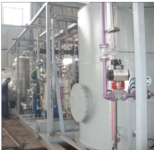
Figure 4—APU constructed for a high SO 3 /acid mist ingress
