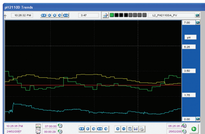
Figure 12—pH and spent electrolyte SCADA trend
