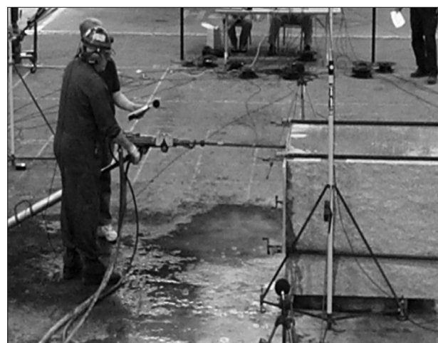
Figure 3—Drilling with the SECO S215
