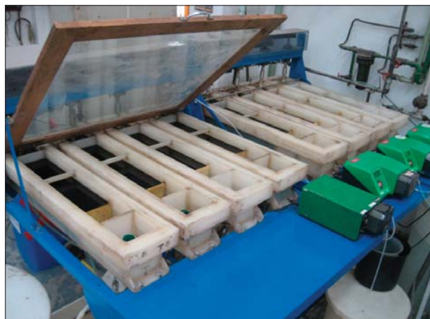
Figure 5c—The integrated pilot plant's solvent extraction units; this versatile plant has eight mixer-settlers that can easily be configured to provide the required number of extraction, washing and stripping stages
