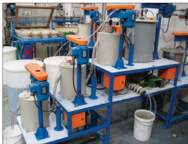
Figure 5a—The integrated plant's bioleach reactors, with the solvent extraction plant in the background: on the right is the feed tank, the dark grey vessel is the 60-litre primary reactor, with three 20-litre reactors arranged in series to the left of that
