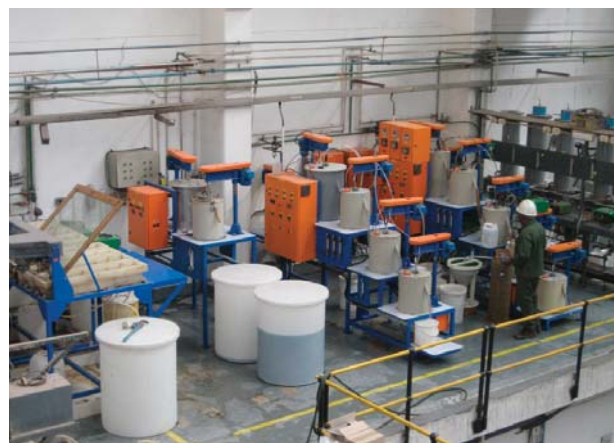
Figure 4—The integrated pilot plant: the solvent extraction plant is on the left, the bioleach pilot plant is in the centre, and the precipitation plant is on the right
