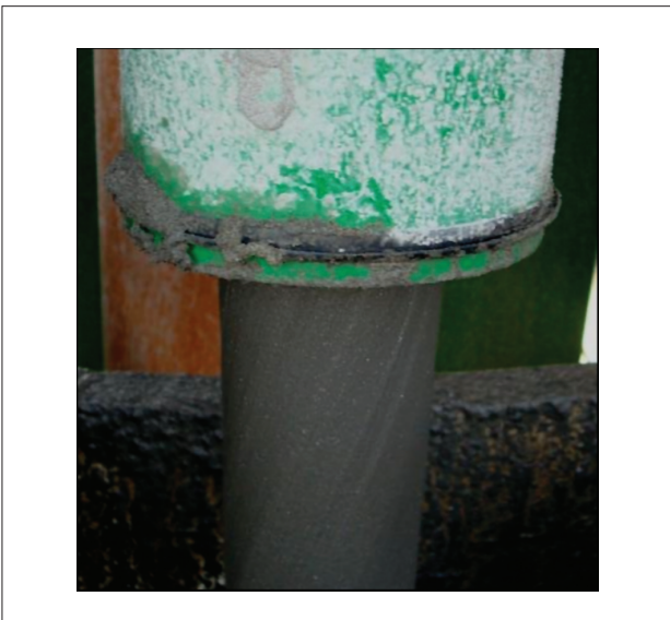
Figure 10—Roping discharge observed at 40% solids concentration, indicating improper use of the hydrocyclone at high solids concentrations
