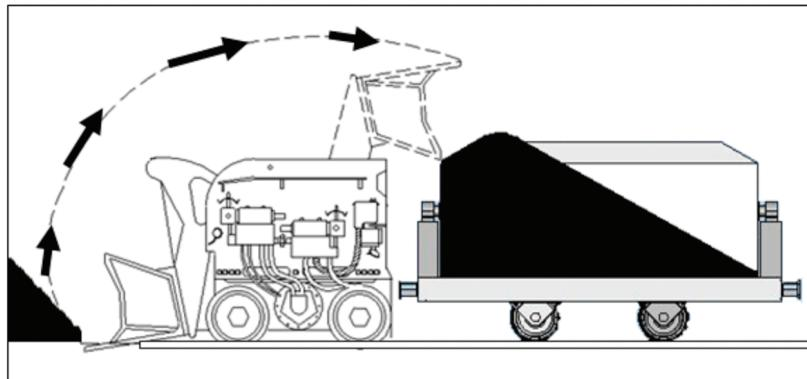
Figure 1—Rocker shovel loading action
