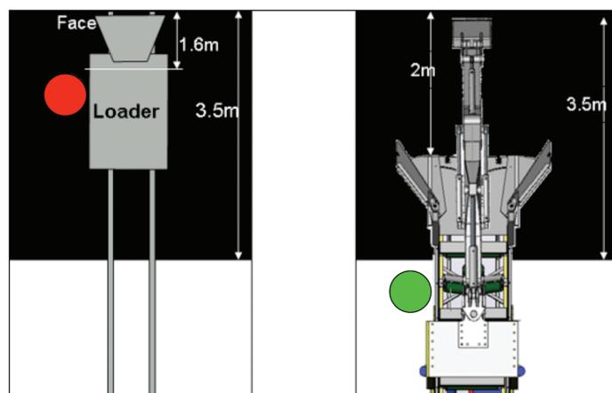
Figure 3—Operator position during loading
