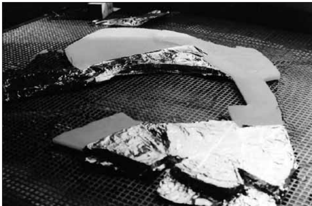
Figure 5—Paraffin block simulating the exploited coal seam within the model
