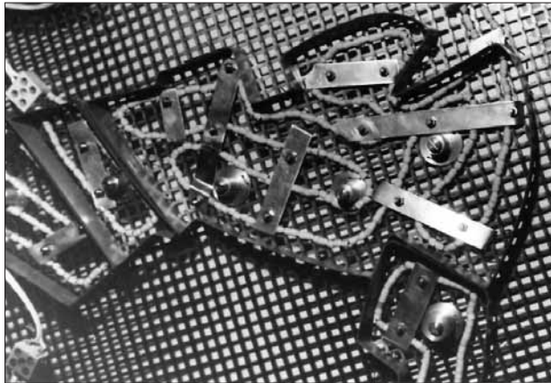
Figure 4—Heating elements (view from below)
