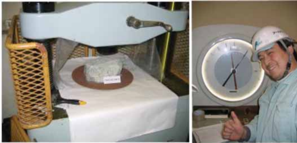
Figure 9—Testing at ECTL Japan, the sample (in shot) required 47 mt force to break, much to the delight of the Japanese 84–100 MPa typical requirement for fracture
