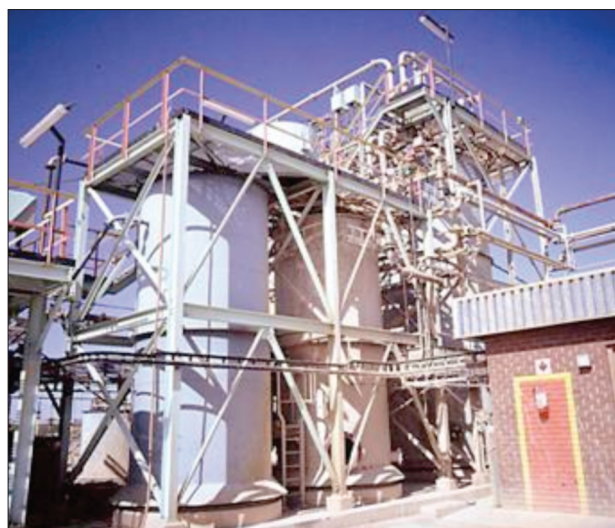
Figure 3—A section of the Vaal Reefs bioleach pilot plant, which was designed to treat 20 t of high-grade pyrite concentrate per day
