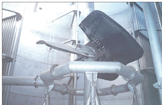
Figure 7—The inside of one of the 700 m 3 bioleach reactors at the Laizhou Bacox™ plant in Shandong, PR China: the octagonal sparger, A-315 impeller and two sets of cooling baffles are all clearly visible
